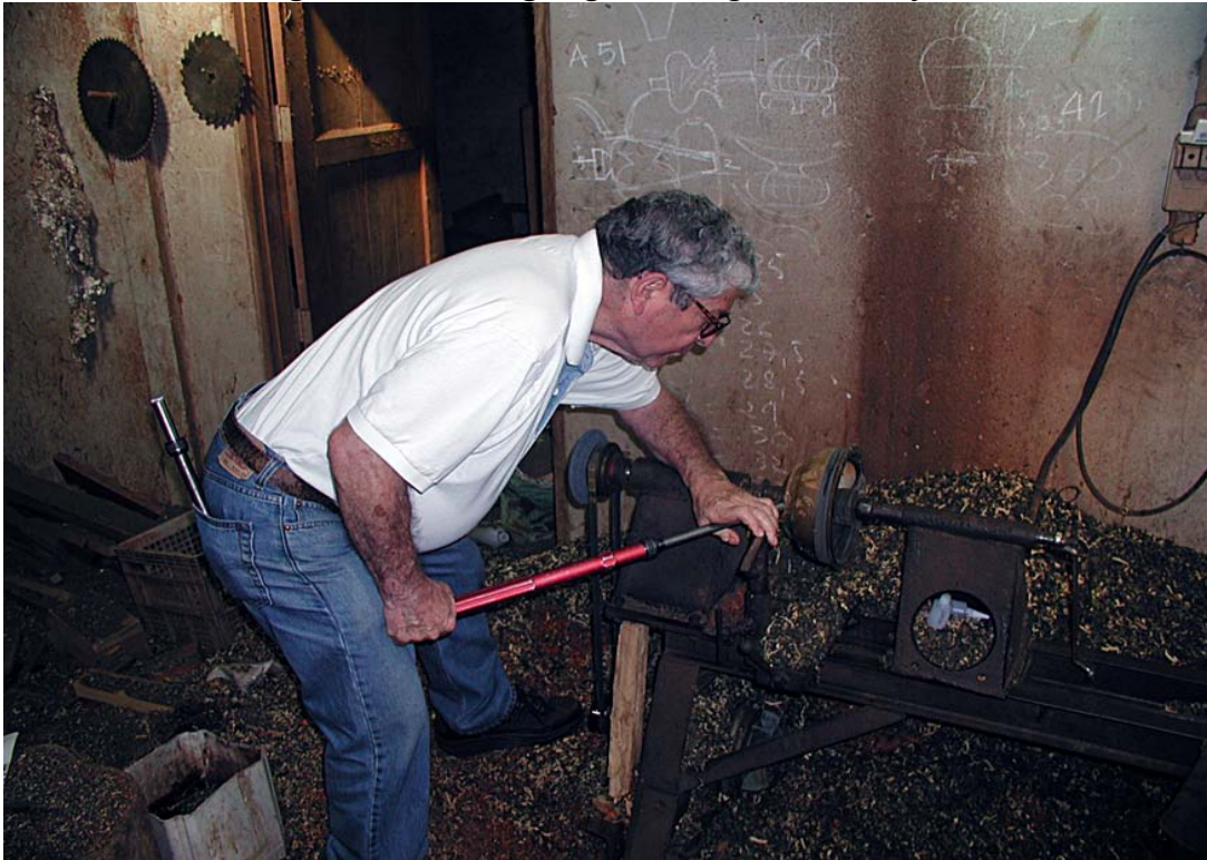
Howie demonstrating the use of a gouge to shape an ebony bowl. Bob's Photos
